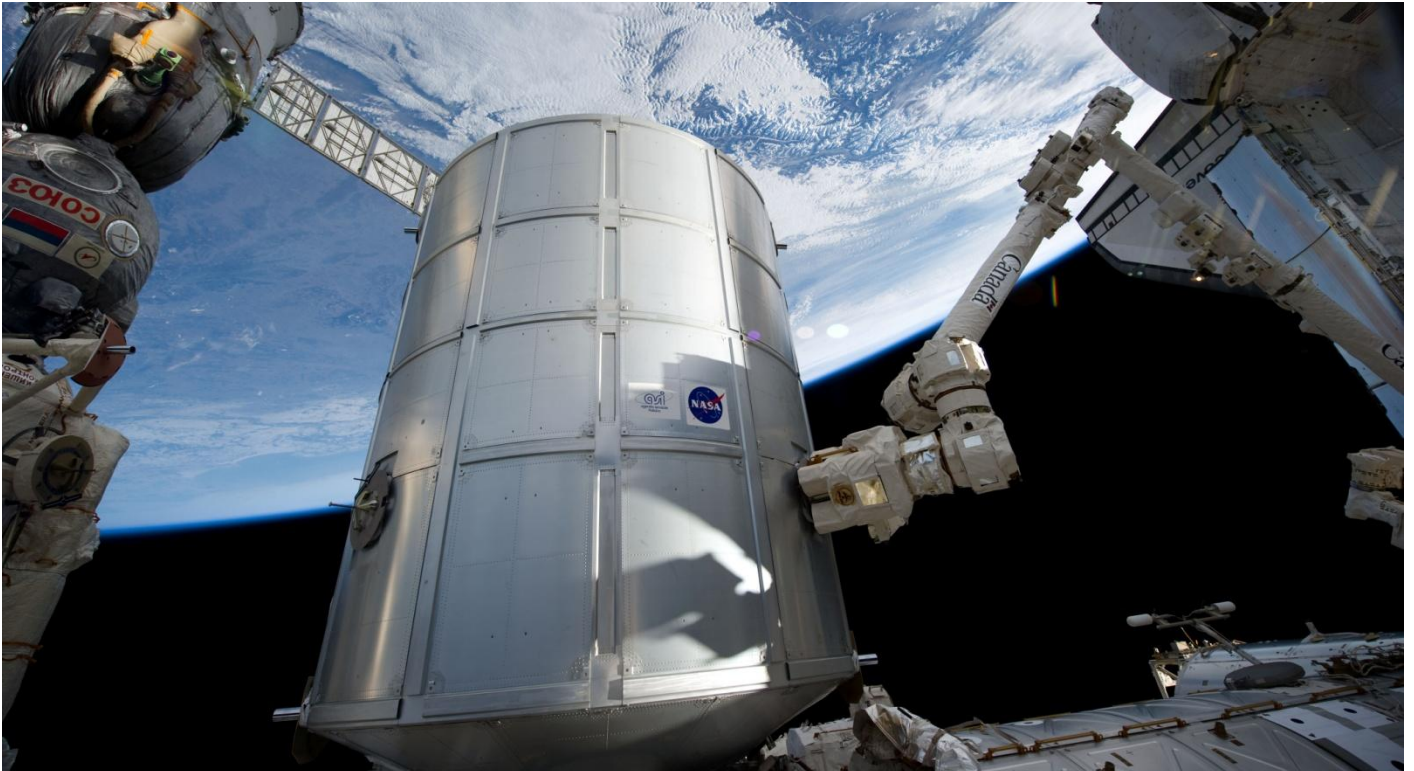
(Bottom) In the grasp of the International Space Station's Canadarm2, the Italian-built Permanent Multipurpose Module (PMM) is transferred from space shuttle Discovery's payload bay to be permanently attached to the Earth-facing port of the station's Unity node. (NASA)
