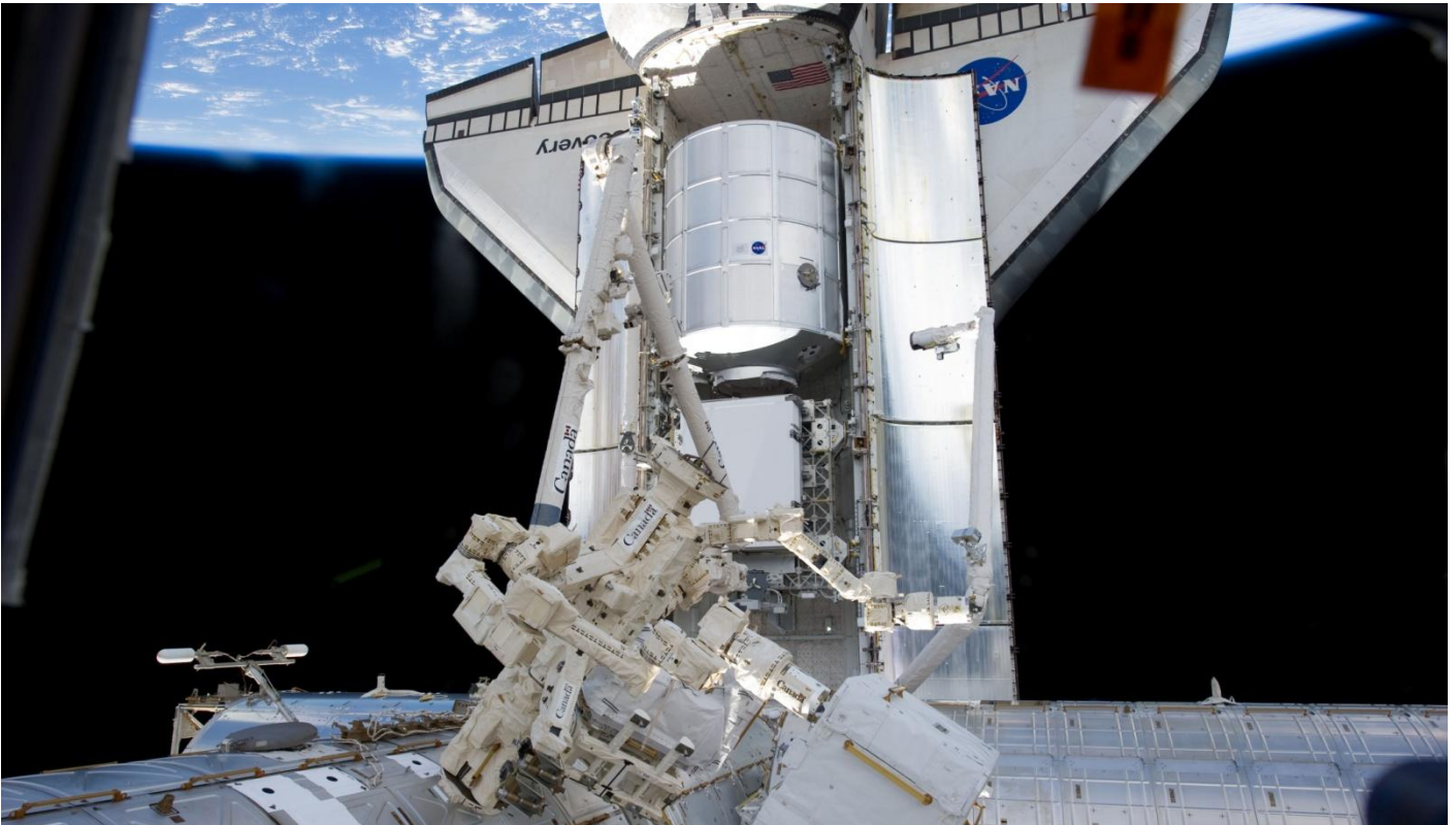
(Bottom) The docked space shuttle Discovery and the Canadian-built Dextre, also known as the Special Purpose Dexterous Manipulator (SPDM), are featured in this image photographed by an STS-133 crew member on the International Space Station. (NASA)
