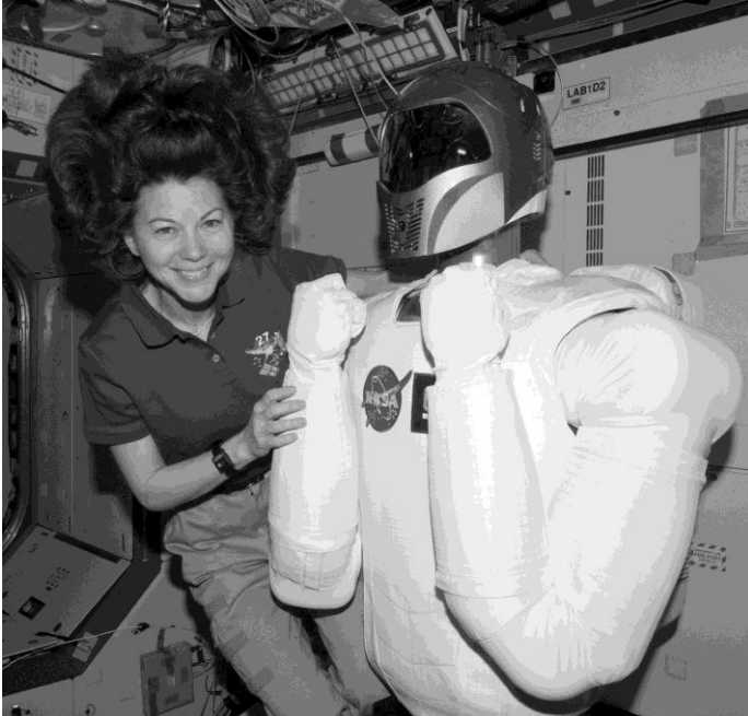
Astronaut Cady Coleman, Expedition 26/27 flight engineer, poses with Robonaut 2, the dexterous humanoid astronaut helper, in the Destiny laboratory of the International Space Station. (NASA)
